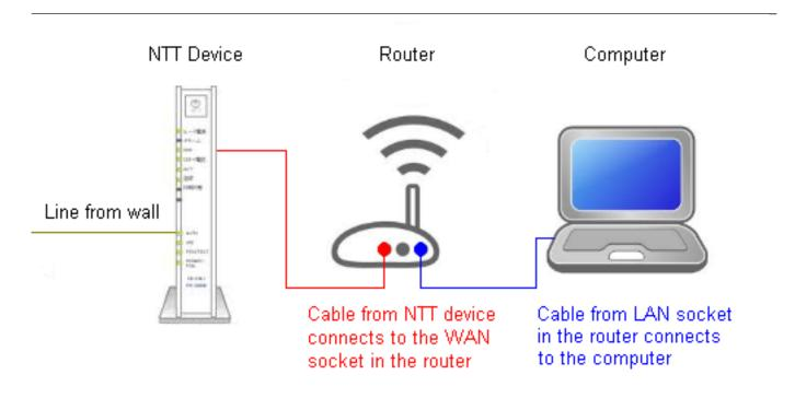
The ethernet cable that comes from the NTT box should go into the WAN/Internet socket on the back of the router. You should then be able to connect the computer to one of the LAN sockets (sometimes labeled as simply numbers, e.g. 1, 2, 3) on the router.
